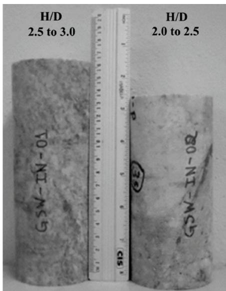
Figure 3 – Example of uniaxial compressive strength rock test samples with two different H/D ratios.
