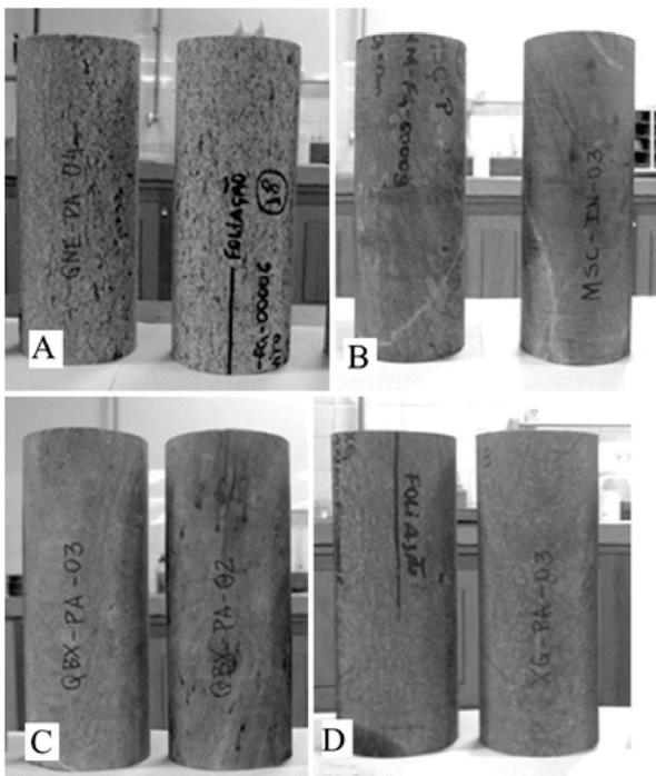
**Figure 1** - Tested lithotypes (a) Granite NE; (b) Silica rich carbonated rock; (c) Quartz Biotite Schist and (d) Graphite rich Schist.
