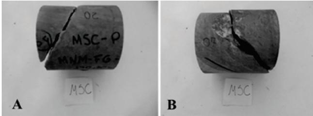
Figure 5 - Example of point load test results considered not valid (a) and valid (b).
