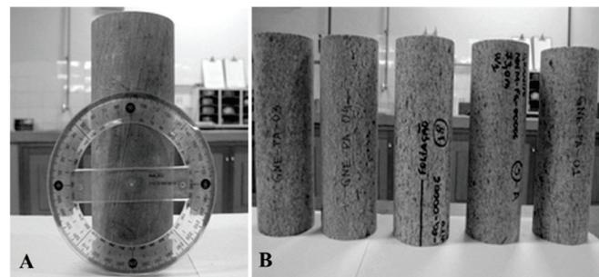
**Figure 2** - Inclination of rock samples tested.
