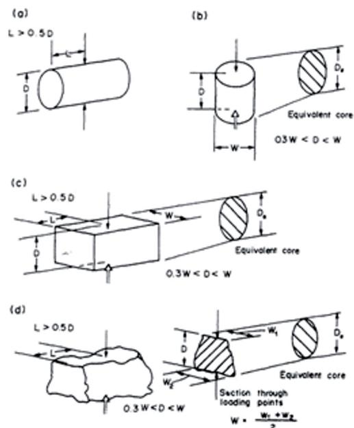
Figure 4 – Rock samples dimensions for point load tests (ISRM 2007).
