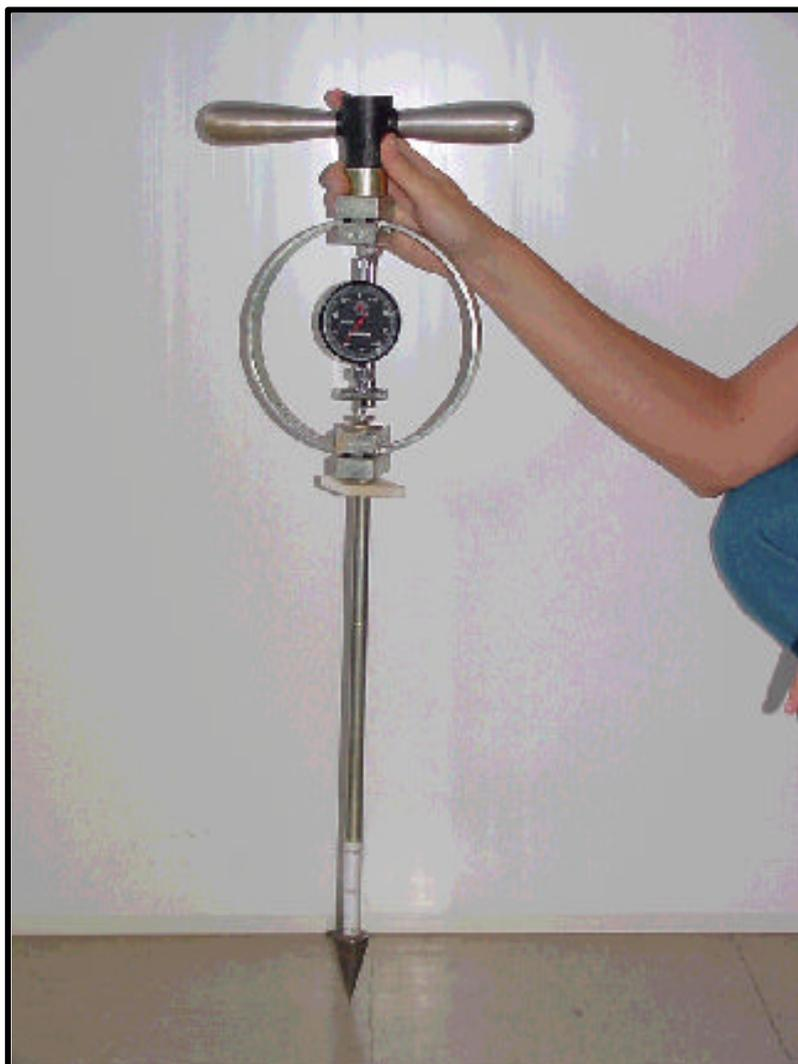
FIGURA 3.3 – Penetrômetro de solos - marca Solotest – ref. 1.210.001
