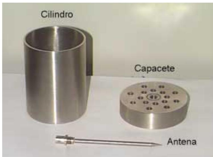
FIGURA 4.10 – Célula coaxial desmontada
