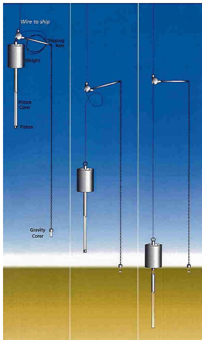
Figura 3-3 Funcionamento do Piston Corer ( http://www.who.edu/instruments/viewInstrument.do?id=8087 ).
