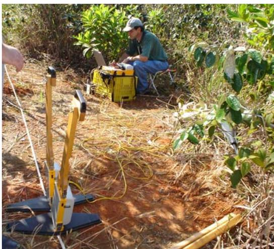
**Arranjo *common offset*** – talude vertical.
