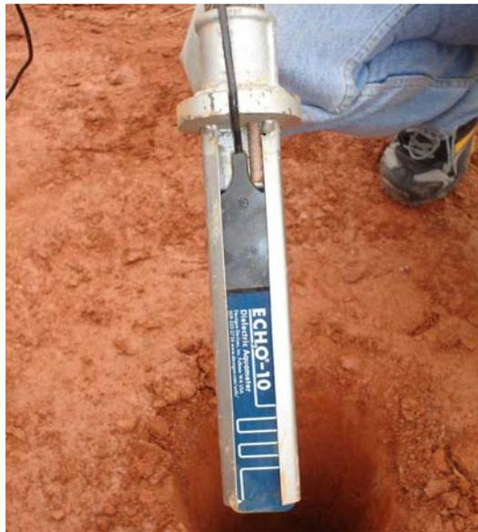
FIGURA 6.22 – SENSOR DE UMIDADE *FDR*.
