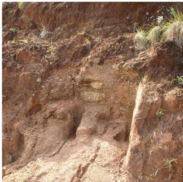
FIGURA 5.4 – COLETA DOS BLOCOS INDEFORMADOS NA ÁREA DO PEREQUÊ-MIRIM.
