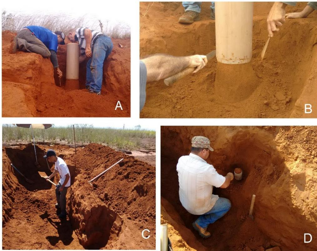
Fig. 3.1 A) Extraction of a large-scale undisturbed soil sample (0.45 m height and 0.20 m inner diameter) from a slope. B) Extraction of a large-scale undisturbed soil sample (0.60 m height and 0.15 m inner diameter). C) Ditch opened to take small-scale samples. D) Extraction of a small-scale undisturbed soil sample (0.15 m height and 0.10 m inner diameter) from the ditch
