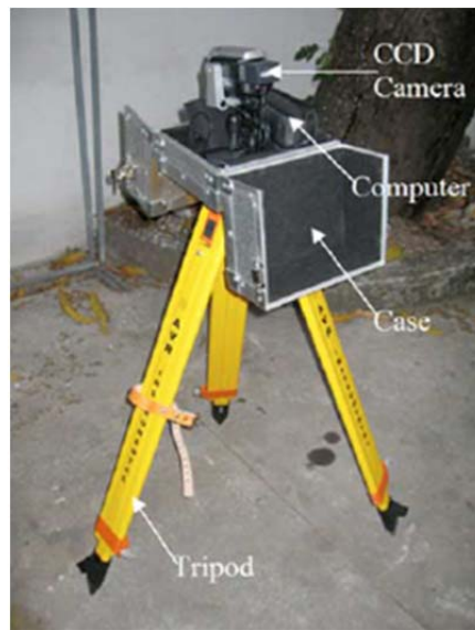
Figura2.19 - O equipamento optical rebound analyzer – PDR (Oliveira et al., 2010).
