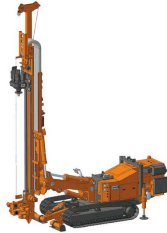
Figura 2.108 Perfuratriz MDT 140B. (MC DRILL TECHNOLOGY, 200-?).
