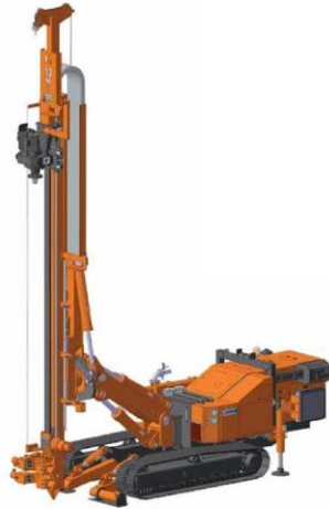
Figura 2.109 Perfuratriz MDT 180B. (MC DRILL TECHNOLOGY, 200-?).
